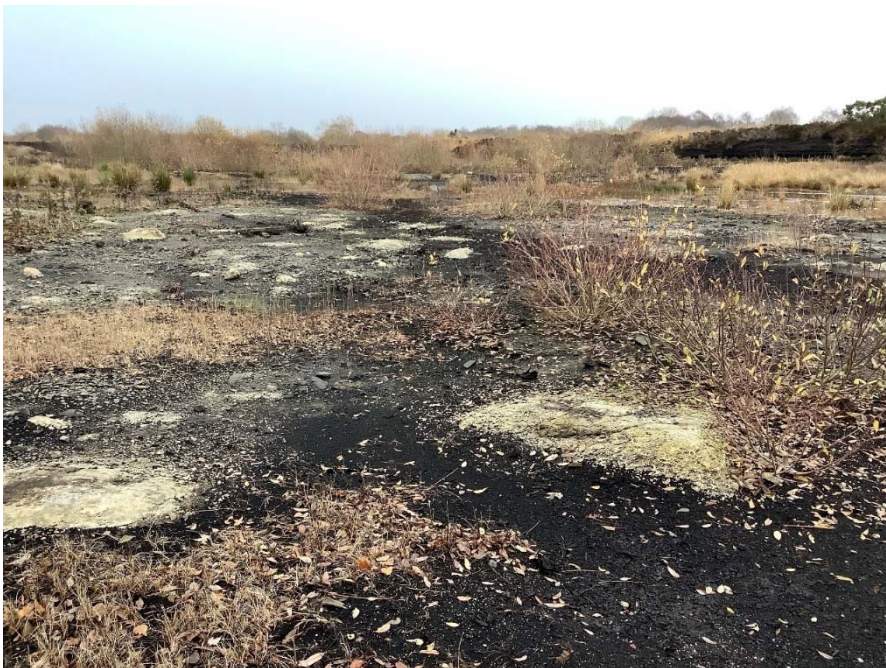
Plate 47: Proposed road to the south of the proposed construction compound looking east. Note dearth of peat in this location. Natural clay exposed in places.
